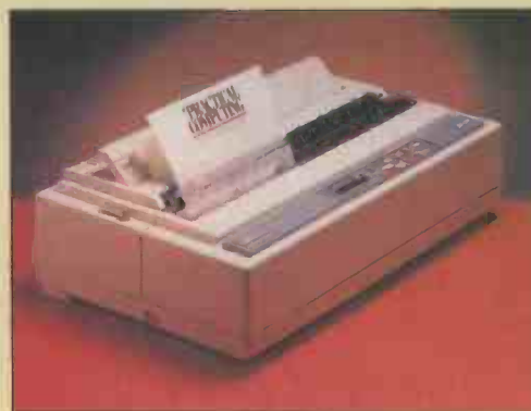
A 132-column carriage is standard on many models, including the Olivetti DM-600.
